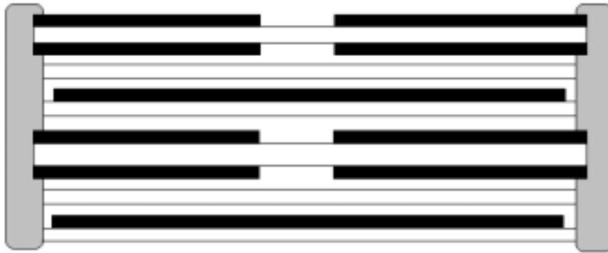
Double-sided metallized electrodes with internal series connections
