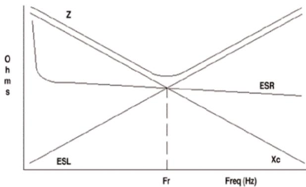
Figure 2. Frequency response characteristics of a capacitor.
